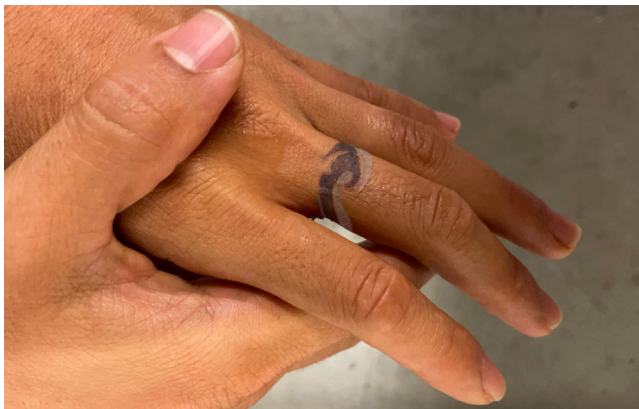
Figure 1: Lotion Interfaces sense and react to applied lotion. Left: “Ocean Waves” ring prototype behaves as a fashionable form of personal expression. Right: “Skyscraper Skyline” prototype extends the display capabilities of a smartwatch onto the skin.
