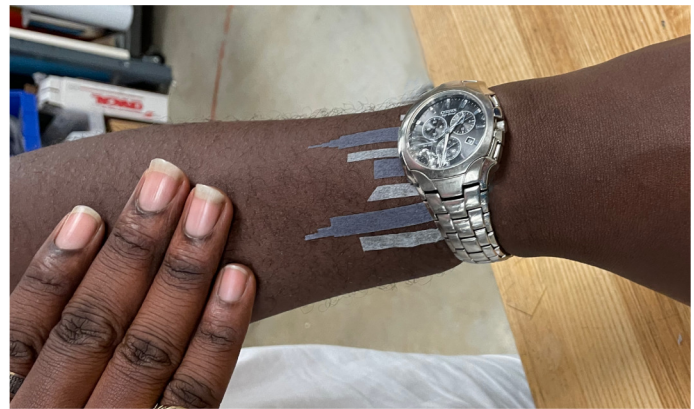
Figure 1: Lotion Interfaces sense and react to applied lotion. Left: “Ocean Waves” ring prototype behaves as a fashionable form of personal expression. Right: “Skyscraper Skyline” prototype extends the display capabilities of a smartwatch onto the skin.
